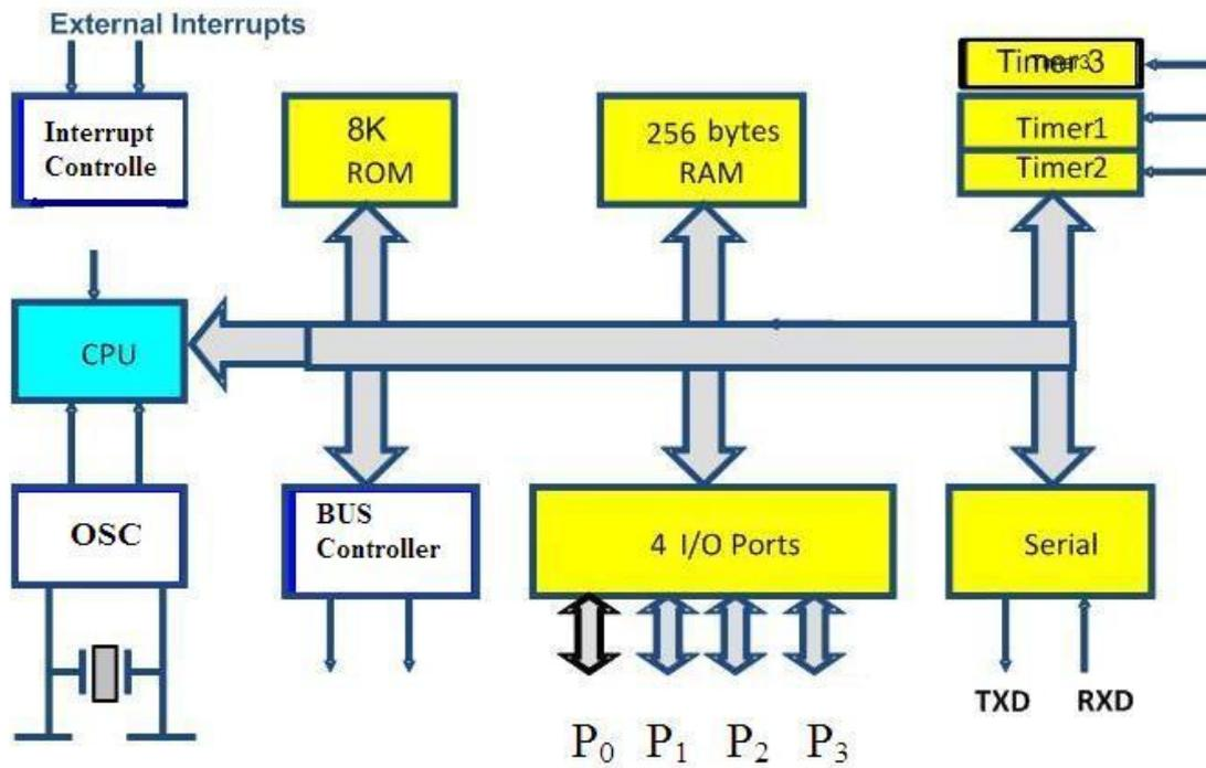
Figure 1 Block diagram of 8052 Hardware Architecture
