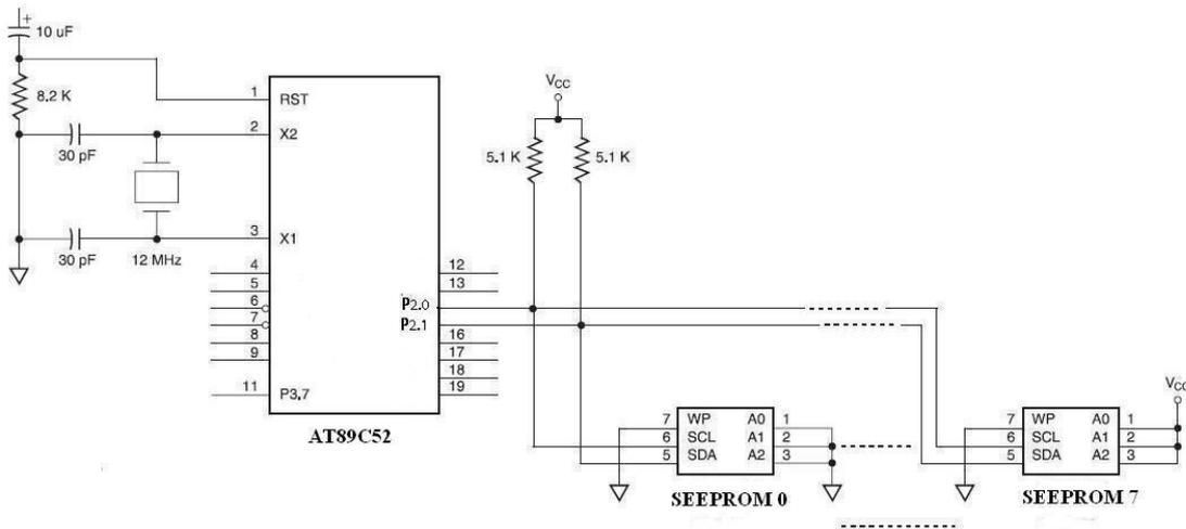
Figure 5 Multi Serial EEPROM( SEEPROM) interfacing
